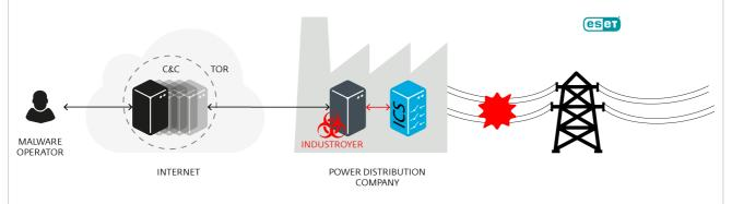
Industroyer is a particularly dangerous threat, since it is capable of controlling electricity substation switches and circuit breakers directly. To do so, it uses industrial communication protocols used worldwide in power supply infrastructure, transportation control systems, and other critical infrastructure systems (such as water and gas).
