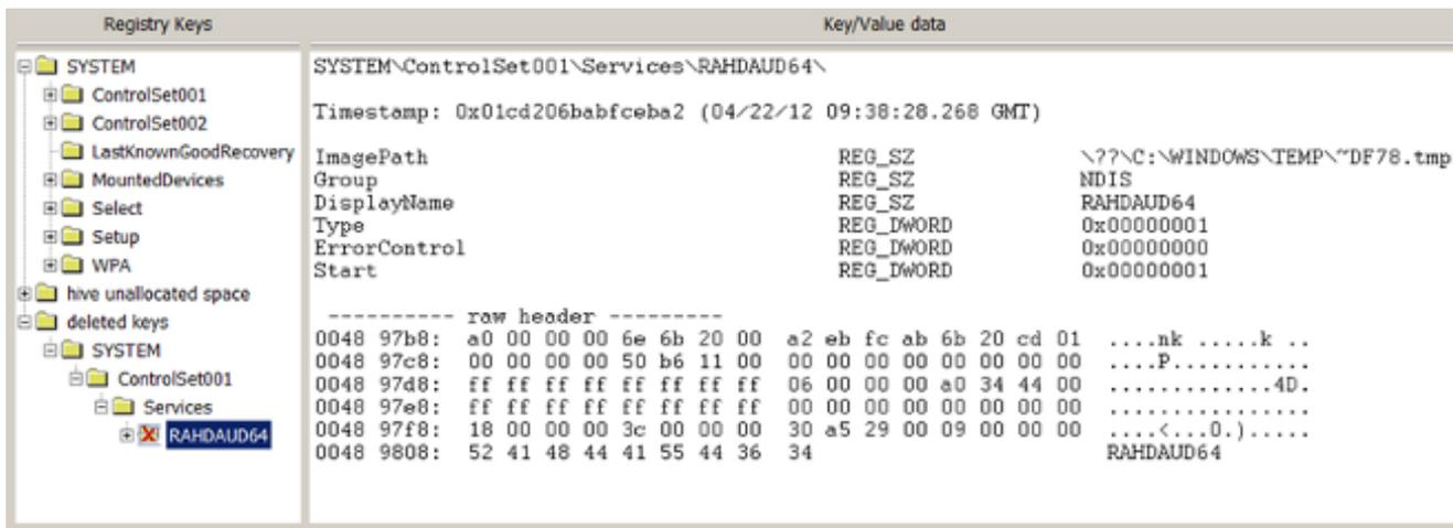
Interestingly, on 22 April, just before this system went down, a specific registry key was created and then deleted. The key was a service named ?RAHDAUD64. It pointed to a file on disk named ?~DF78.tmp, in the ?C:\WINDOWS\TEMP folder.
