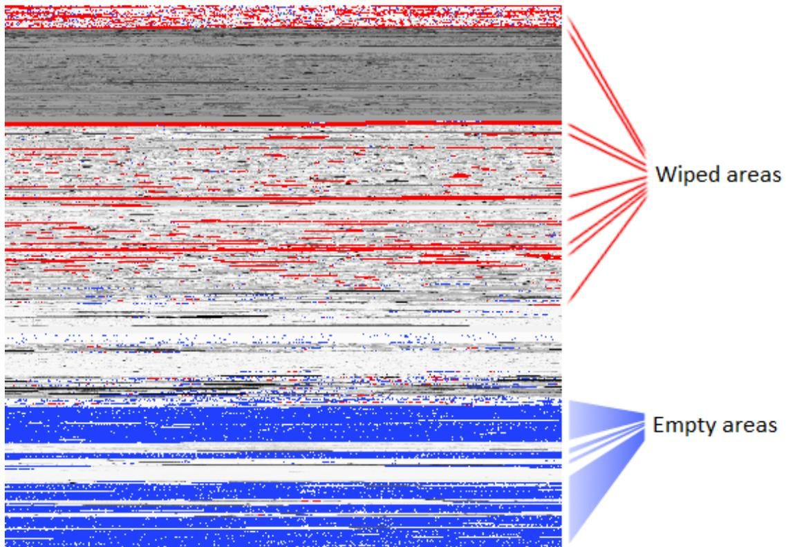
As you can see, Wiper managed to do a pretty good job of destroying most of the disk. One can observe a red-filled stripe at the top which indicates an area that has been cleaned well. Although no clear pattern is visible, a large amount of the disk has been filled with unusable data. The wiping operation obviously focused on the beginning of the disk, then it affected the middle of the disk, before the system finally crashed.
